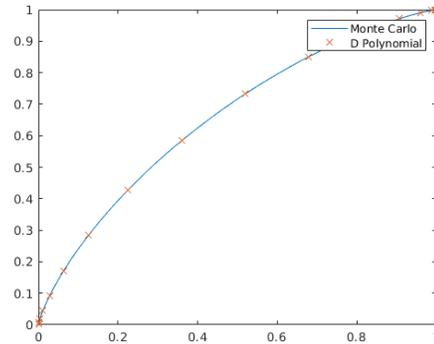
Fig. 3.  $P_f$  vs  $P_d$  computed using exact expressions for  $F_{\lambda_1}(x)$  calculated using equation (4) and a Monte Carlo simulation with  $10^6$  trials for  $M = 4$  and  $N = 10^5$  with  $-15$  dB per channel SNR
