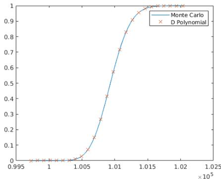
Fig. 2. Comparison of  $F_{\lambda_1}(x)$  calculated using equation (4) and a Monte Carlo simulation with  $10^6$  trials for  $M = 4$  and  $N = 10^5$  with  $-15$  dB per channel SNR
