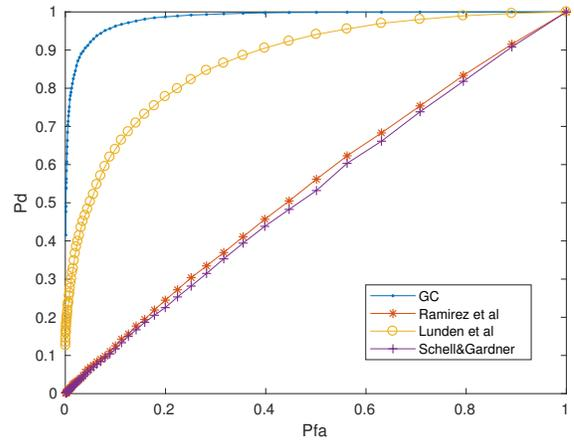
Fig. 3. ROC curves for CS vs. WGN,  $M = 4$ ,  $\text{SNR} = -20\text{dB}$
