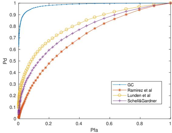
Fig. 2. ROC curves for CS vs. WGN,  $M = 3$ ,  $\text{SNR} = -16\text{dB}$
