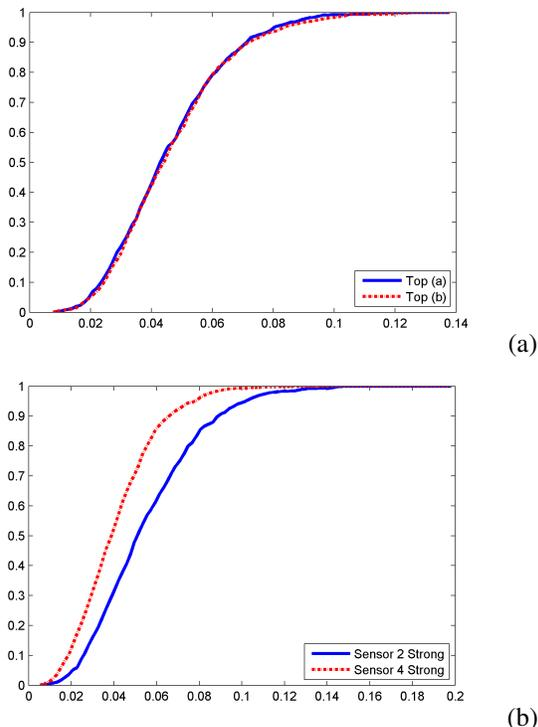
**Fig. 5.** (a) Empirical cumulative distribution functions obtained under the null hypothesis for the two distinct network topologies with four nodes and four edges. (b) Empirical CDFs obtained with various SNRs on the four nodes.
