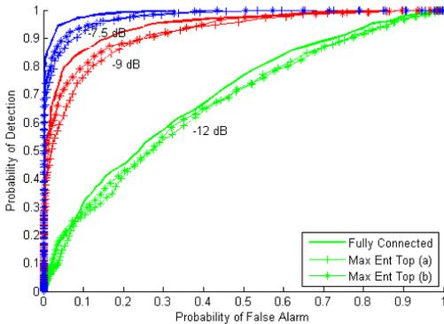
**Fig. 3.** ROC curves for detection in complete and surrogated four-node networks at three different SNRs.
