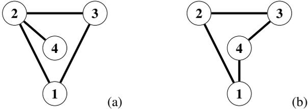
**Fig. 2.** The two distinct topologies for a four-node network with four edges.
