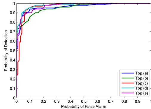
**Fig. 4.** ROC curves for detection in complete and surrogated twenty-node networks at three different SNRs. Maximum-entropy matrix completion in this case was accomplished numerically via convex optimization.
