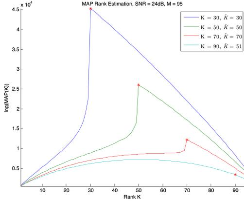
**Fig. 2.** MAP estimate results for  $M = 95$ ,  $N = 100$ ,  $K = 30, 50, 70, 90$  for the blue, green, red and cyan lines respectively, with an SNR at the receiver of 24dB. The red asterisk represents the point where the true rank falls on the MAP. Each line represents a single iteration.
