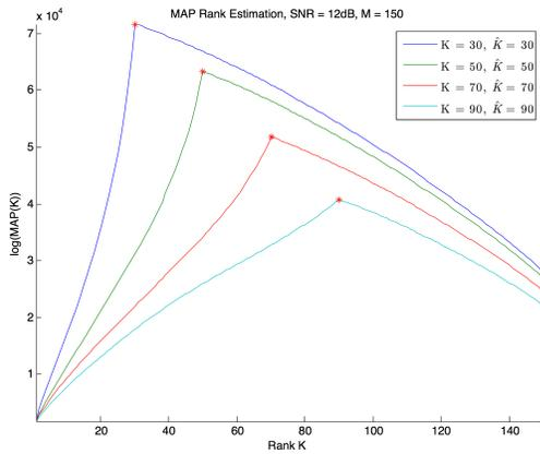
**Fig. 3.** MAP estimate results for  $M = 150$ ,  $N = 200$ ,  $K = 30, 50, 70, 90$  for the blue, green, red and cyan lines respectively, with an SNR at the receiver of 12dB. The red asterisk represents the point where the true rank falls on the MAP. Each line represents a single iteration.
