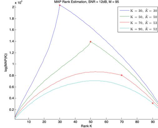
**Fig. 1.** MAP estimate results for  $M = 95$ ,  $N = 100$ ,  $K = 30, 50, 70, 90$  for the blue, green, red and cyan lines respectively, with an SNR at the receiver of 12dB. The red asterisk represents the point where the true rank falls on the MAP. Each line represents a single iteration.
