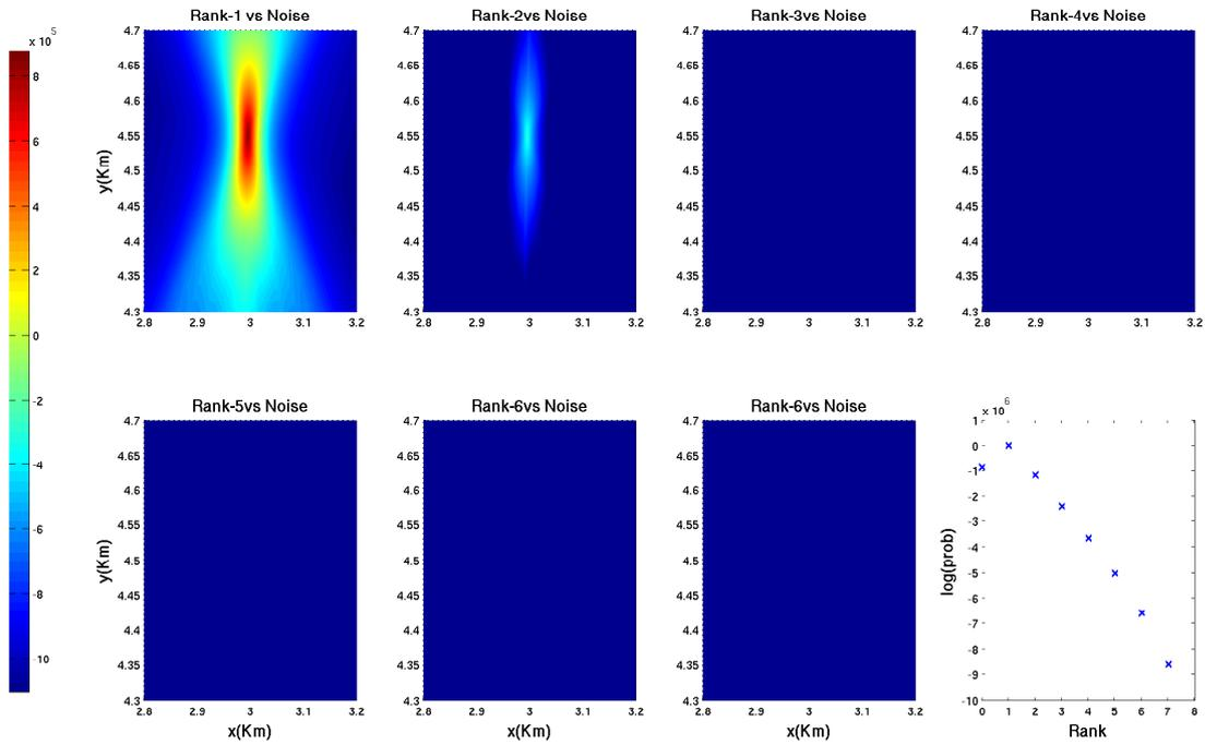
Fig. 4. Plots of likelihood ratio between the rank- $K$  signal hypothesis  $H_K$ ,  $K = 1, \dots, 7$ , and the noise-only hypothesis  $H_0$  for a rank-1 (conventional) phased array radar signal.
