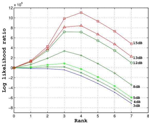
Fig. 2. Log-likelihood ratio values for the hypothesized signal rank  $K = 1, \dots, 7$  at different SNRs.
