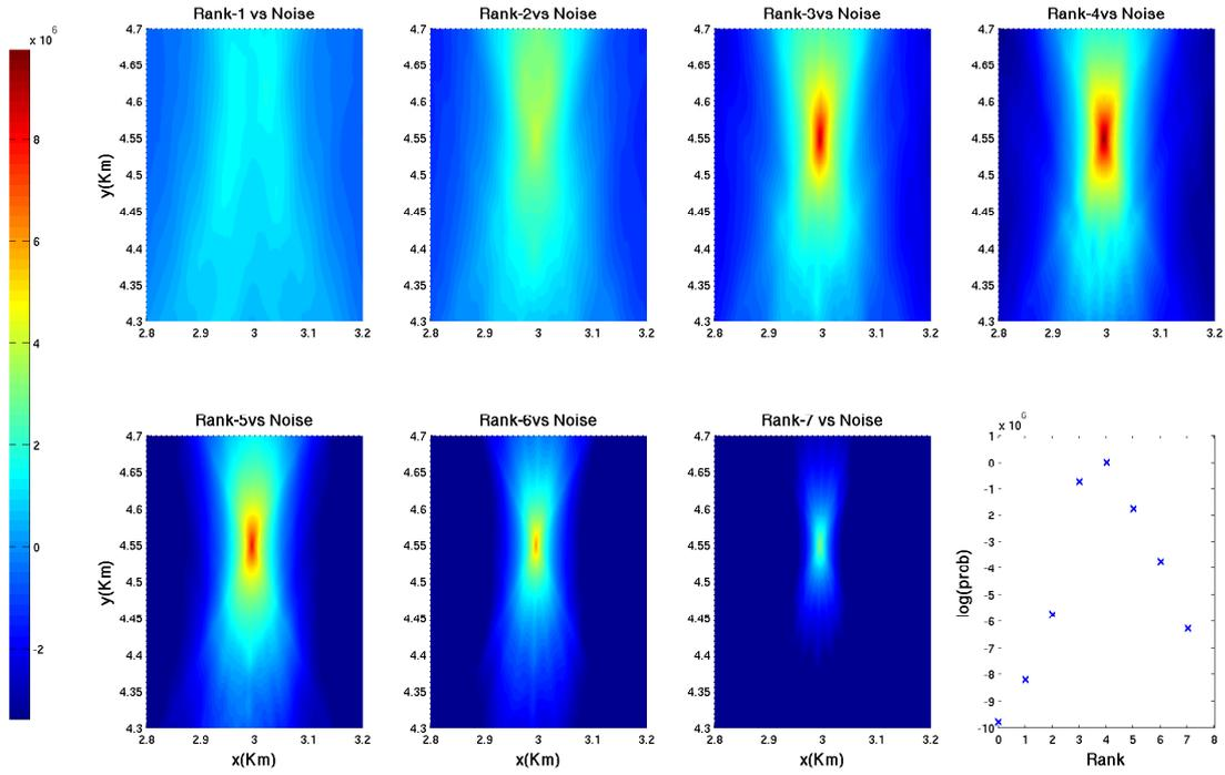
Fig. 3. Plots of likelihood ratio between the rank- $K$  signal hypothesis  $H_K$ ,  $K = 1, \dots, 7$ , and the noise-only hypothesis  $H_0$  for a rank-4 (MIMO) phased array radar signal.
