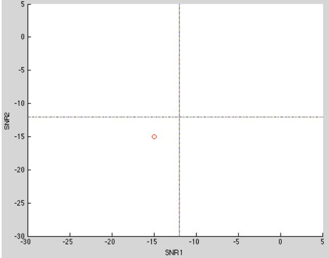
**Fig. 3.** SNRs on two receiver channels needed to achieve  $P_f = 0.1$  and  $P_d = 0.9$  for infinite SNR on one channel. The dashed lines show the SNR values (in dB) on one receiver channel required to achieve this performance level with the matched filter. The marked point shows the equal-channel SNR required to achieve this performance with a three-channel coherence detector with a noiseless signal replica on one channel and using  $\lambda_{\max}$  as the detection statistic.
