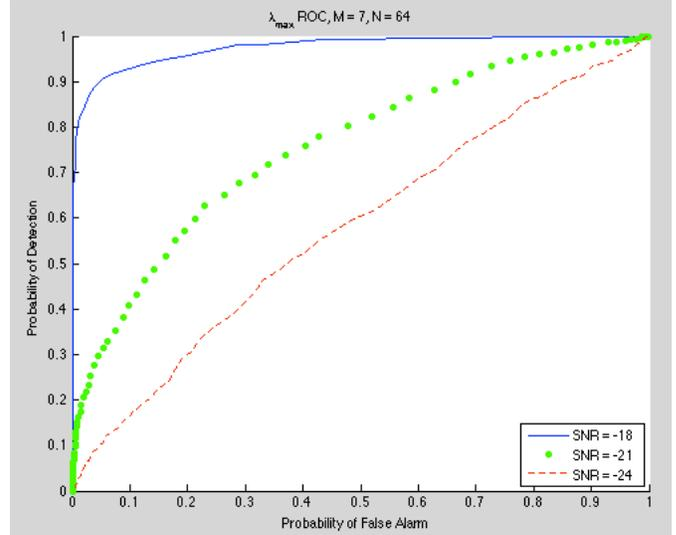
**Fig. 4.** Detection probability ( $P_d$ ) versus false alarm probability ( $P_f$ ) for a seven-channel largest eigenvalue detector with sequence length  $N = 64$ . Channel one contains a noiseless signal replica, while the remaining six channels have equal SNR values. The solid line represents an SNR of -18dB, the dotted line represents an SNR of -21dB, and the dashed line represents an SNR of -24dB.
