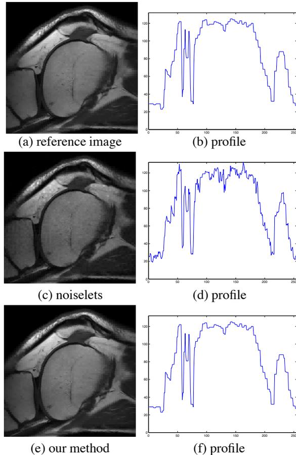
**Fig. 3.** (a)  $256 \times 256$  knee 10%-sparse image. (c) reconstructed image with noiselet, error = -22 dB. (e) reconstructed image with our method. The error is much smaller, -284 dB. The respective horizontal slices in (b), (d), and (f) also show our result is identical to the reference image.
