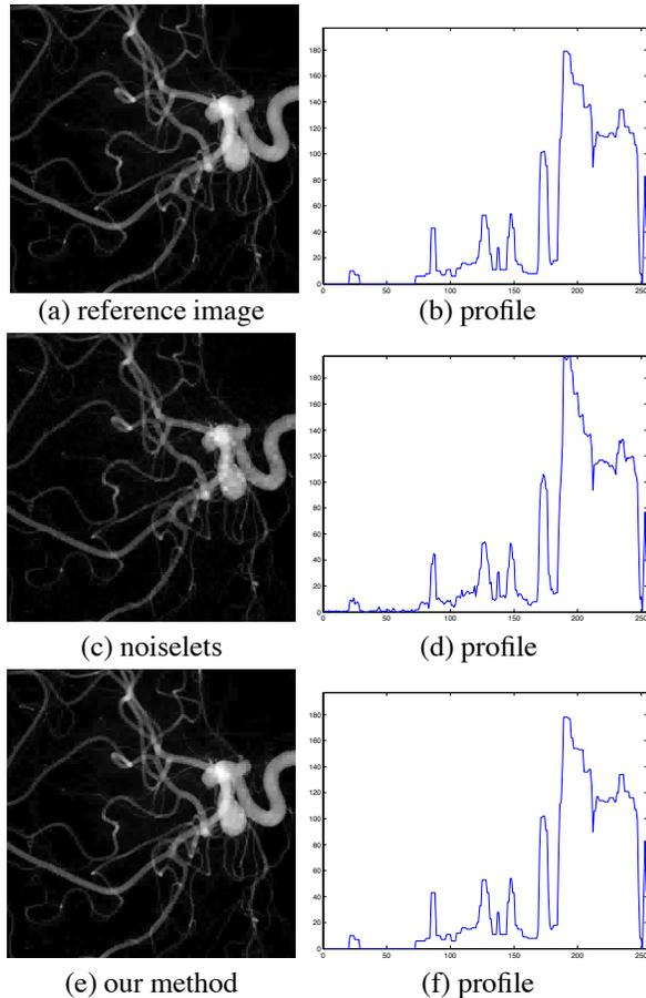
**Fig. 2.** (a)  $256 \times 256$  vessel image with 10% sparsity. (c) reconstructed image with noiselets, error is -19 dB. (e) reconstructed image with our method, whose error is smaller, -283 dB. The respective horizontal slices in (b), (d), and (f) also show our result is identical to the reference image.
