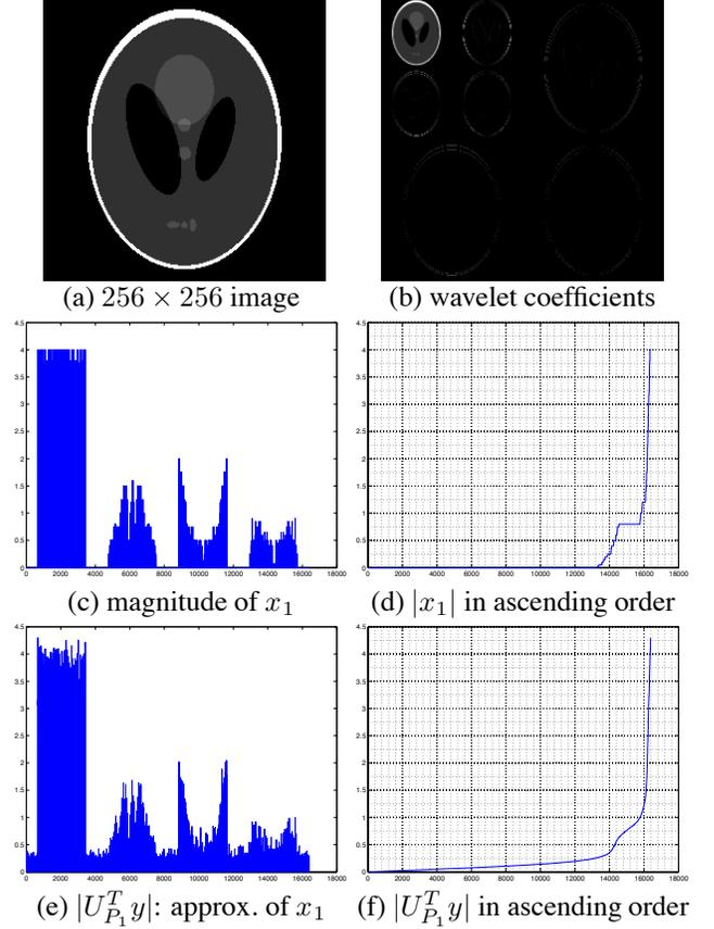
**Fig. 1.** In (b) it is shown that the energy of wavelet coefficients is concentrated in the upper-left region; in (c) and (e) it is shown that  $|U_{P_1}^T y|$  approximates  $|x_1|$  well; (d) is the plot of  $|x_1|$  sorted in ascending order, and finally, (f) is  $|U_{P_1}^T y|$  in ascending order.
