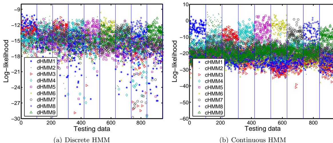
Figure 5. Log-likelihood of the testing data computed by the trained HMMs with “dHMM” denoting “discrete HMM” and “cHMM” denoting “continuous HMM”.
