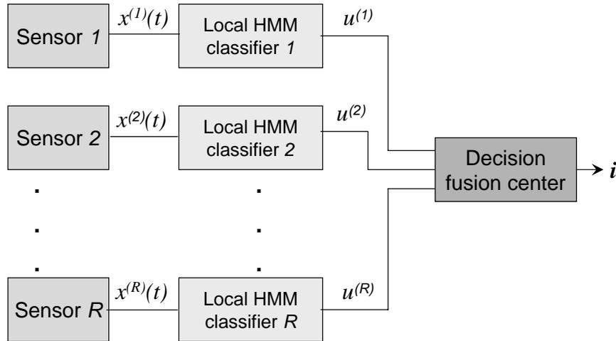
Figure 1. Block diagram of the sensor fusion algorithm using method 1.
