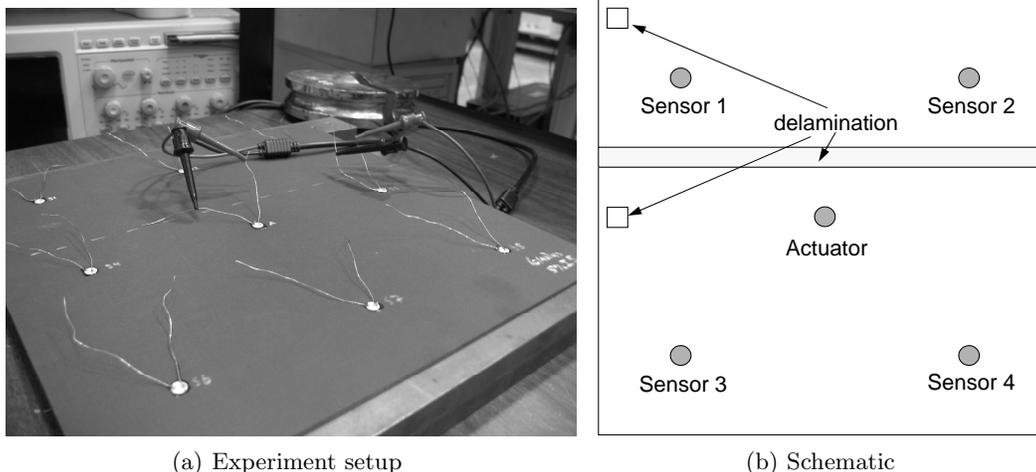
Figure 3. Experimental setup for delamination damage in a 292.1 mm  $\times$  292.1 mm laminated composite with 5% delamination, and schematic showing the delamination and sensor layout.
