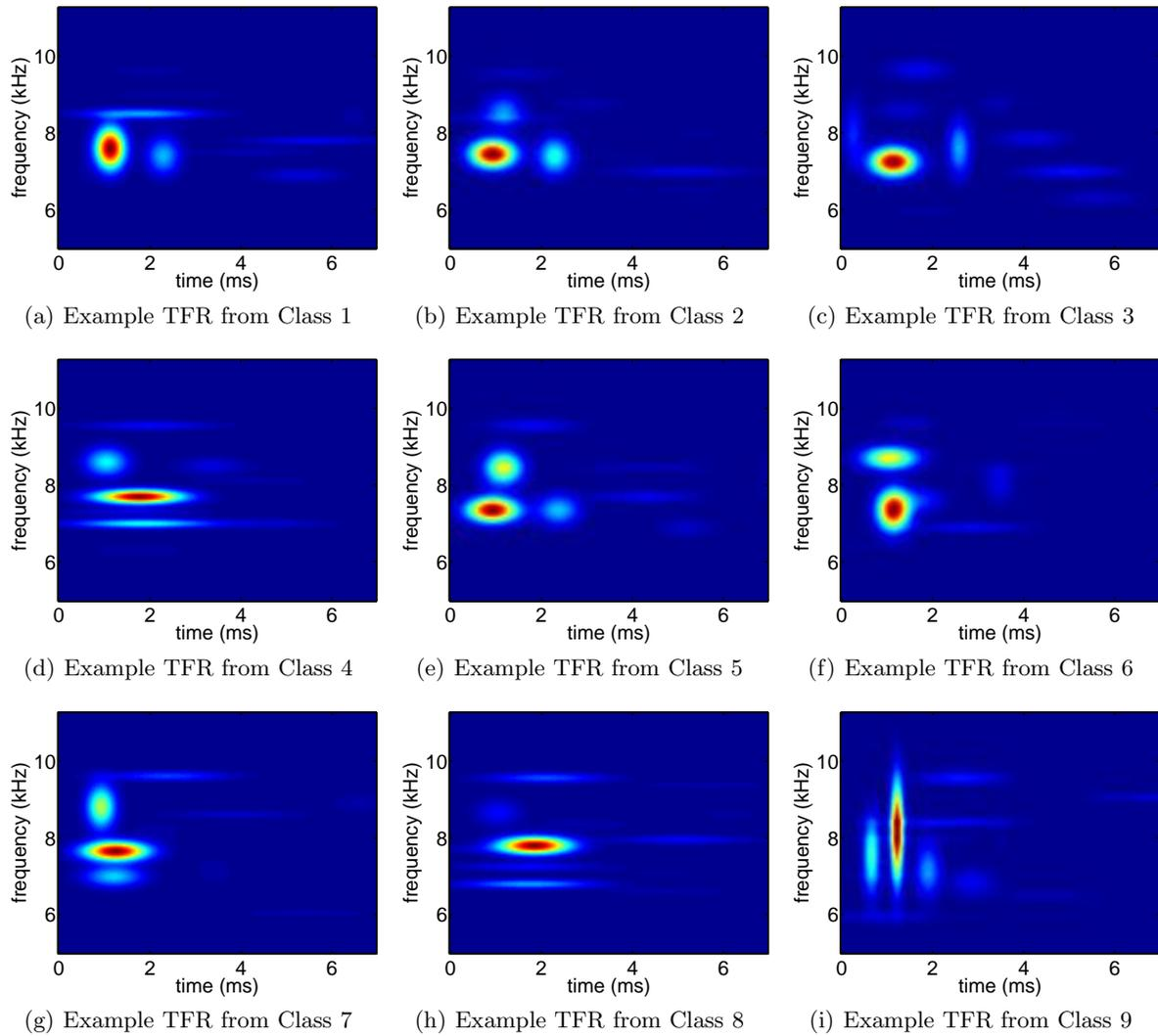
Figure 4. Example TFR plots from all 9 damage classes using recorded waveforms from PZT 3
