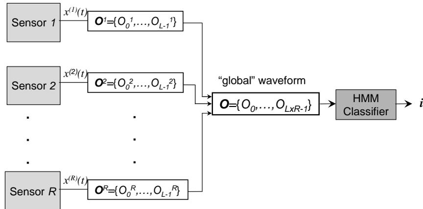
Figure 2. Block diagram of the sensor fusion algorithm using method 2.
