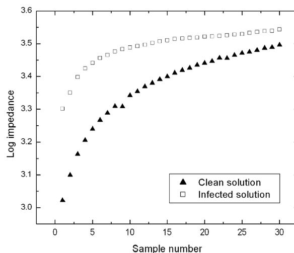
**Fig. 2.** Logarithmic impedance curves for clean and infected solutions (volume of  $100 \mu\text{l}$ ) over time (represented by discrete sample numbers). The samples represent impedance values at time  $T = 10 \times (\text{sample number})$  seconds. The difference between the clean and infected solutions is significant.
