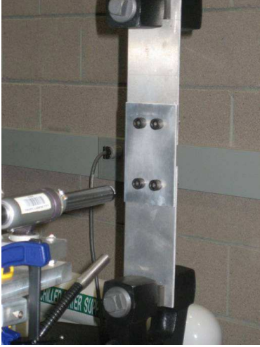
Fig. 2. Setup for structural and material damage in a bolted joint.
