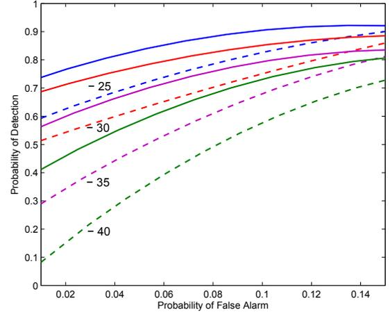
**Fig. 2.** ROC curves with different SCR values. The numbers indicate SCR values in dB. Dashed lines are ROC curves using a fixed LFM chirp (without waveform design); solid lines are ROC curves using proposed dynamic method (with waveform design).
