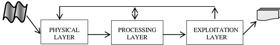
Figure 2. Integration of sensing and processing via feedback.
