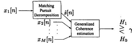
Figure 2: Block diagram of the GC detector that utilizes the MPD algorithm. Here,  $x_1[n]$  is assumed to be the output of the highest SNR channel, and  $\hat{s}[n]$  is the MPD estimate.
