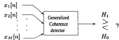
Figure 1: Multiple channel GC detector.
