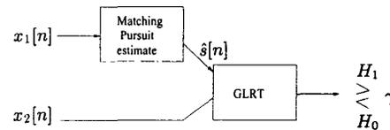
Figure 3: Block diagram of the GLRT detector using two channels that utilizes the MPD estimate,  $\hat{s}[n]$ .
